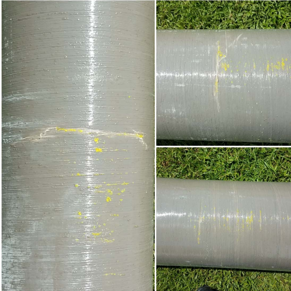
Photo 4 – Typical Failure of Fortress Pilings – Single Lateral Crack at Reaction #2
