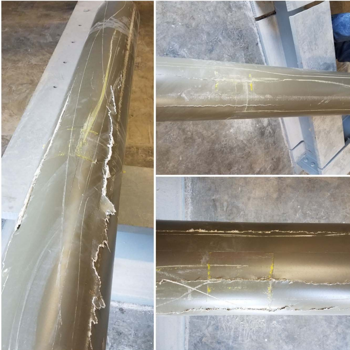
Photo 5 – Typical Failure of Superpile – Longitudinal Cracking from P to Reaction #2
